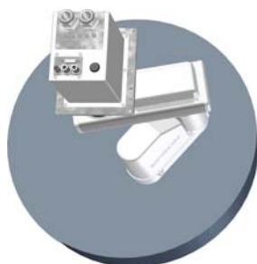
Epson Spider: cylindrical envelope without dead space
