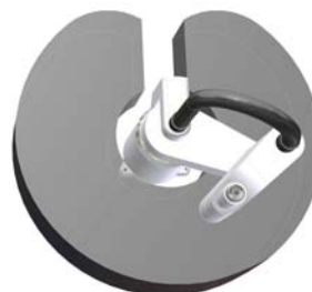
SCARA robots: kidney-shaped envelope with dead space
