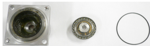
Reduction gear Wave generator O-ring
